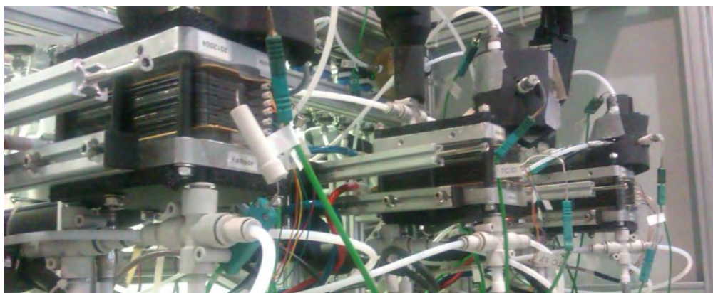
FIGURE 1 Long-term parallel operation of three short stacks.
