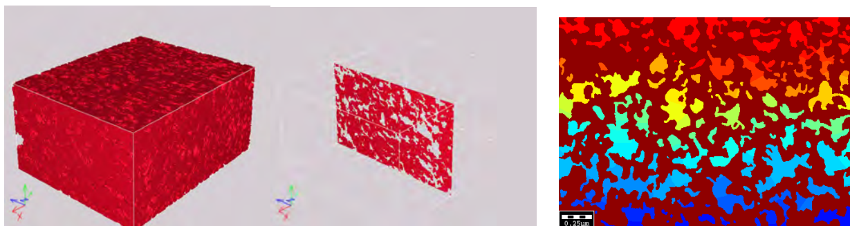
Figure: Left: 3D structure of a catalyst layer, reconstructed from FIB/SEM images[3]. Right: diffusion in the catalyst layer pores: numerically determined concentration distribution.
